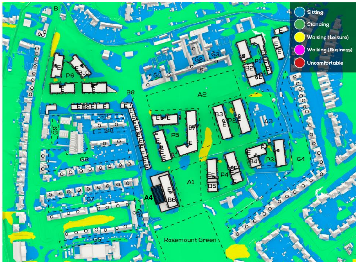
Figure 15 10 Ground Level Summer Comfort for Operational Phase
