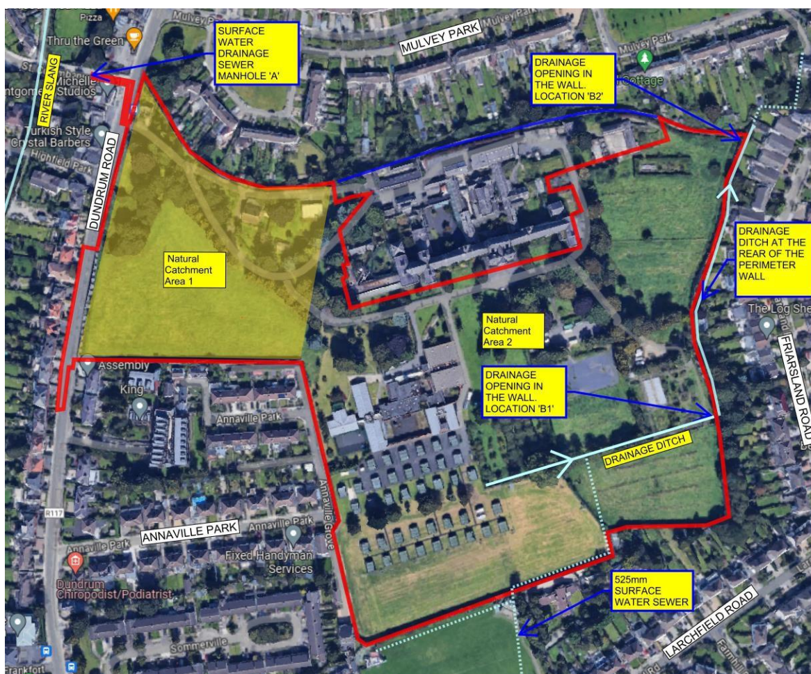
Figure 10.2 Aerial view of the site with water drainage indicated (Source: BMCE, 2024)
